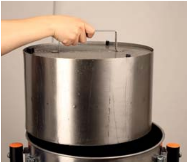
Removing the demister cassette.
