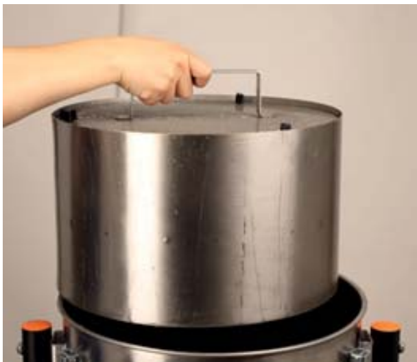
Removing the demister cassette.
